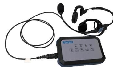
The noise reduction device (80 x 130 x 30 mm) commercialized using the voice recognition system. It is used together with a headset.
